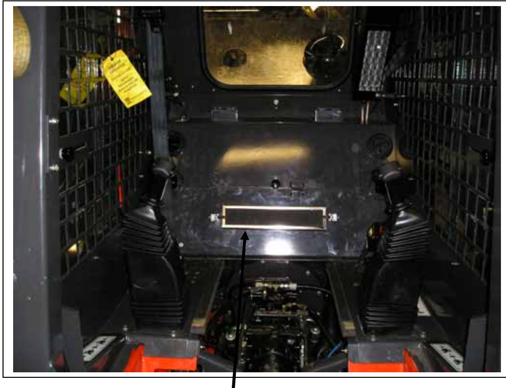
Filter and clips in place
