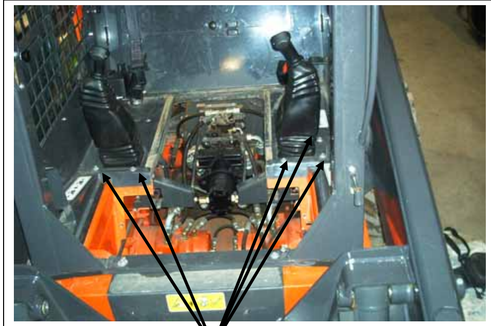
Screws fastening the control arm boot.
