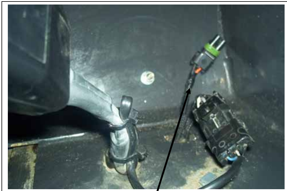
Seat belt wiring harness
