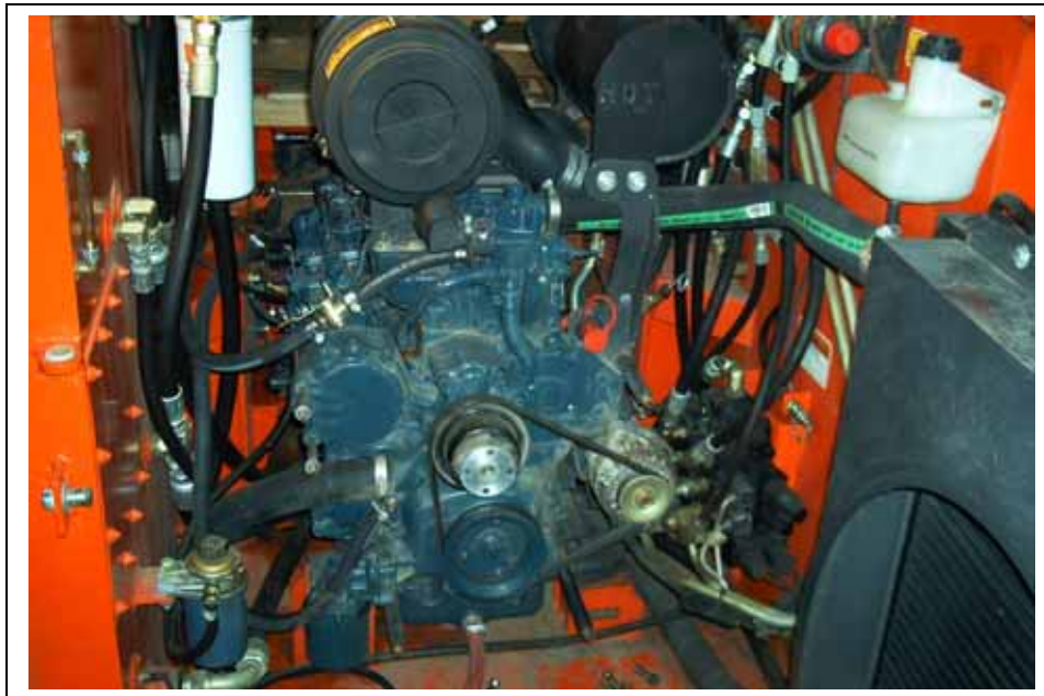
Engine compartment with fan and guard removed.
