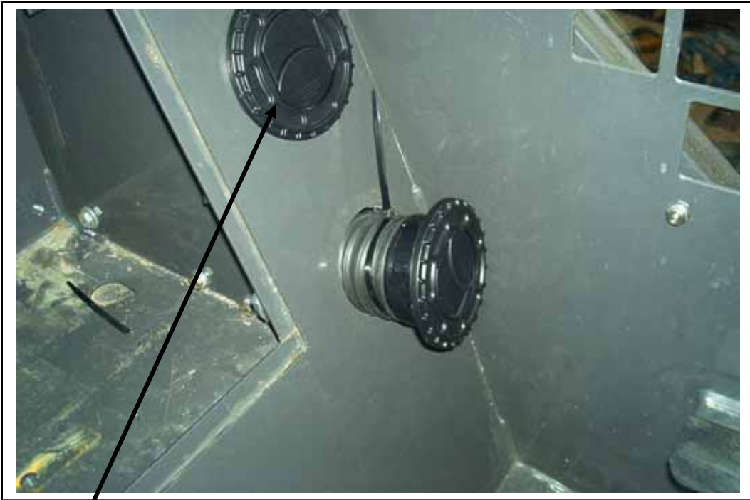
The 2 upper louvers are no longer required here. They are now located on the top of this shelf to supply the upper ducting.
