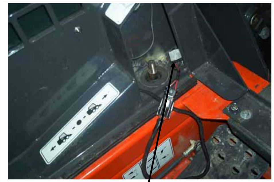
Wiring harness out the bottom of column
